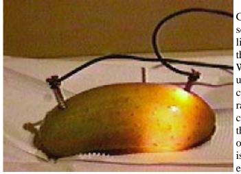
Currents in ionic solutions are often not linearly proportional to the applied voltage. When <u>Ohm's law</u> is used with ordinary carbon resistors, the ratio of voltage to current is constant, but the variation in light output suggests that this is not the case with the electric pickle.
