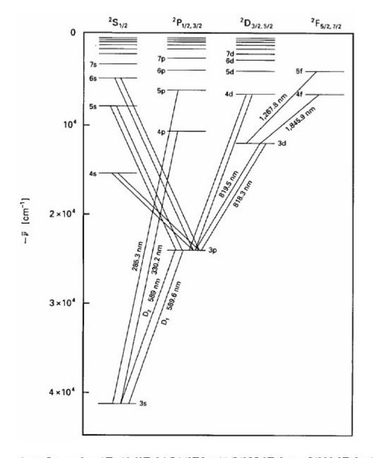
4p to 5p: to 3s ;  $\Delta E = (6.63E-34 \text{ Js})(3E8 \text{ m/s})(1/285.3E-9 \text{ m} - 1/330.2E-9 \text{ m}) = 9.48E-20 \text{ J}$ 4f to 5f: to 3d ;  $\Delta E = (6.63E-34 \text{ Js})(3E8 \text{ m/s})(1/1267.8E-9 \text{ m} - 1/1845.9E-9 \text{ m}) = 4.91E-20 \text{ J}$ 3d levels: to 3p  $\Delta E = (6.63E-34 \text{ Js})(3E8 \text{ m/s})(1/818.3E-9 \text{ m} - 1/819.5E-9 \text{ m}) = 3.56E-22 \text{ J}$
