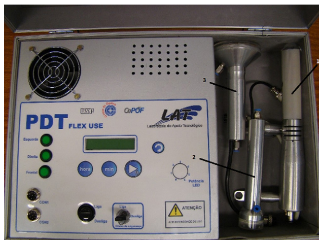
Fig. 1 The homemade device “PDT Flex Use”. This portable system consists of a briefcase containing three probes with different sizes: 1 – a cylinder for intravaginal illumination; 2 – a smaller circular device for external illumination of minor warts; 3 – a larger circular probe for illumination of lesions with an average diameter of 5 cm.
