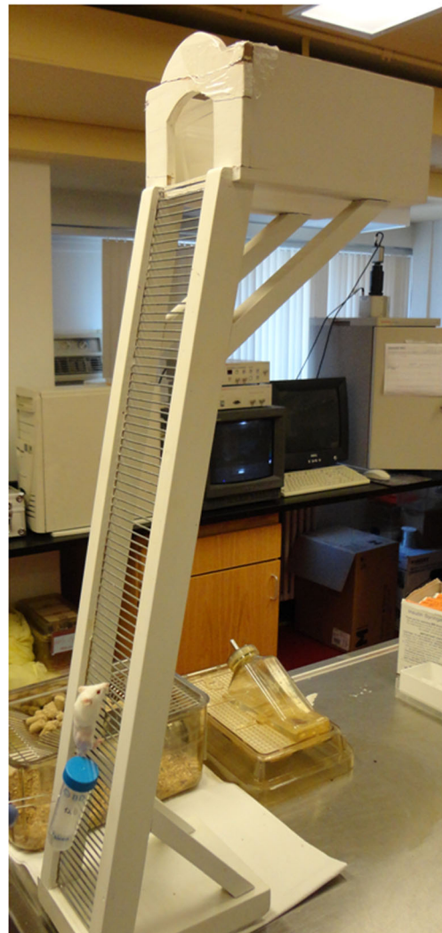
Fig. 2 Ladder. Inclined ladder (80°) with 100×9 cm (length and width, respectively) used for the fatigue test. Falcon tube filled with water and attached to mouse tail
