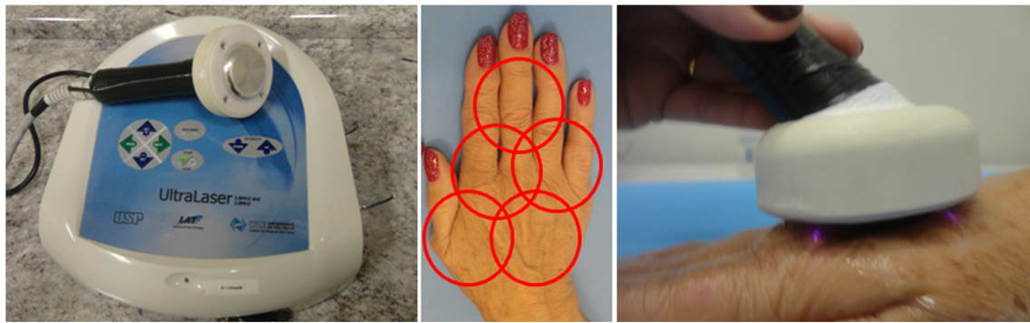
Fig. 1 Prototype with four diode laser beams around one US transducer, points of application on the hand, and US plus laser during therapeutic session
