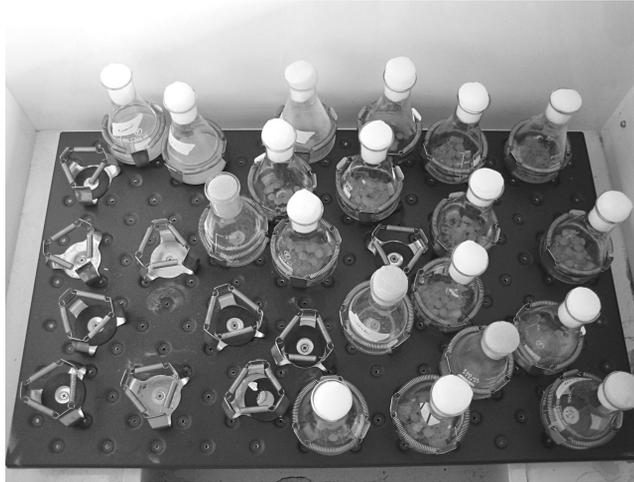
**Figure 8.8** *Single stage flat bed shaking incubator (Photo: Michelle Lea, John Moores University, Liverpool)*
