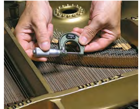
A technician uses a micrometer to measure the diameter of a piano wire. (Courtesy of Buck Rogers/Craftsmen Piano Rebuilders North Attleboro, MA.)
