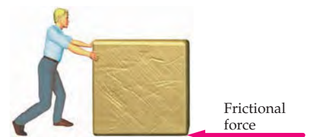
FIGURE 4-8 The man is pushing on a block. The frictional force exerted by the floor on the block opposes its sliding motion or its tendency to slide.
