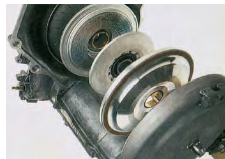
The rotating plates in the transmission of a truck make inelastic collisions when engaged. (Dick Luria/FPG International.)
