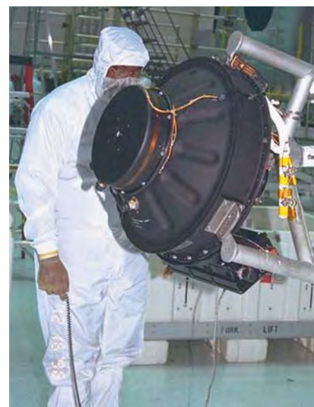
An astronaut examines the reaction wheel of the Hubble Space Telescope. (NASA/Goddard Space Flight Center.)
