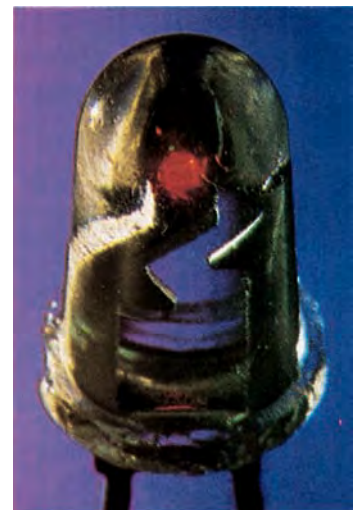
A light-emitting diode (LED). (© C. Falco/Photo Researchers.)
