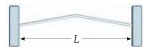
FIGURE 16-22 A string plucked at the center. When it is released, its vibration is a linear superposition of standing waves.
