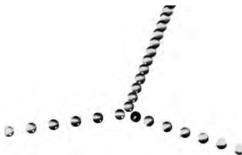
Multiframe photograph of an off-center elastic collision of two balls of equal mass. The dotted ball, entering from the left, strikes the striped ball, which is initially at rest. The final velocities of the two balls are perpendicular to each other. (Berenice Abbot/Photo Researchers.)
