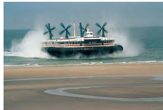
Friction is greatly reduced by a cushion of air that supports the hovercraft. (Jose Dupont/Explorer/Photo Researchers.)
