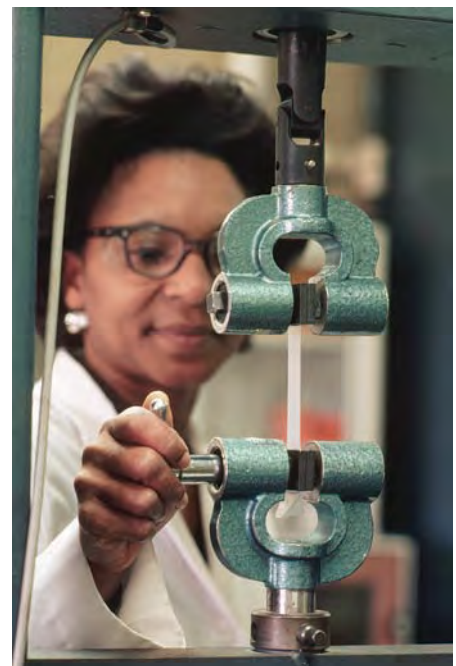
To measure the tensile strength, the rod is stretched until it breaks. (Vince Streato/CORBIS.)
