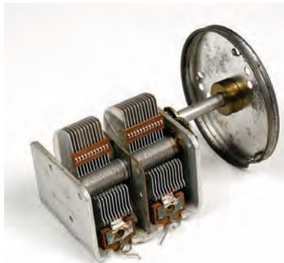
A variable air-gap capacitor such as those used in the tuning circuits of old radios. The semicircular plates rotate through the fixed plates, which changes the amount of surface area between the plates, and hence the capacitance. ( Loren Winters/Visuals Unlimited. )
