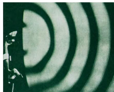
Sound waves from a telephone handset spreading out in the air. The waves have been made visible by sweeping out the space in front of the handset with a light source whose brightness is controlled by a microphone. (From Winston E. Kock, Lasers and Holography , 1978, Dover Publications, New York.)
