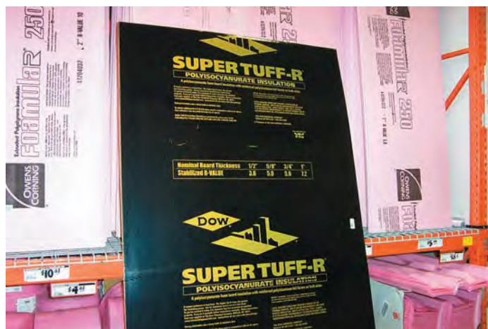
FIGURE 20-12 For a 1-in. thickness of this material, the R_f = 7.2 . (Courtesy of Eugene Mosca.)
