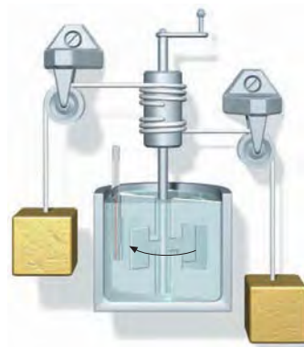
FIGURE 18-2 Schematic diagram for Joule's experiment. Insulating walls surround water. As the weights fall at constant speed, they turn a paddle wheel, which does work on the water. If friction is negligible, the work done by the paddle wheel on the water equals the loss of mechanical energy of the weights, which is determined by calculating the loss in the potential energy of the weights.
