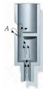
FIGURE 16-19 Cutaway view of a section of a flue-type organ pipe. Air is blown against the edge, causing a swirling motion of the air near point A that excites standing waves in the pipe. There is a pressure node near point A , which is open to the atmosphere.
