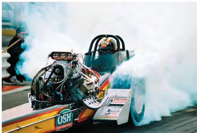
An exhaust manifold feeds the header pipes seen on this top-fuel dragster in order for the engine to release heat and reduce its temperature. (© 2002 Robert Briggs.)
