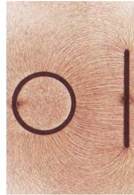
Electric field lines for an oppositely charged cylinder and plate, shown by bits of fine thread suspended in oil. Note that the field lines are normal to the surfaces of the conductors and that there are no lines inside the cylinder. The region inside the cylinder is electrically shielded from the region outside the cylinder. (Harold M. Waage.)
