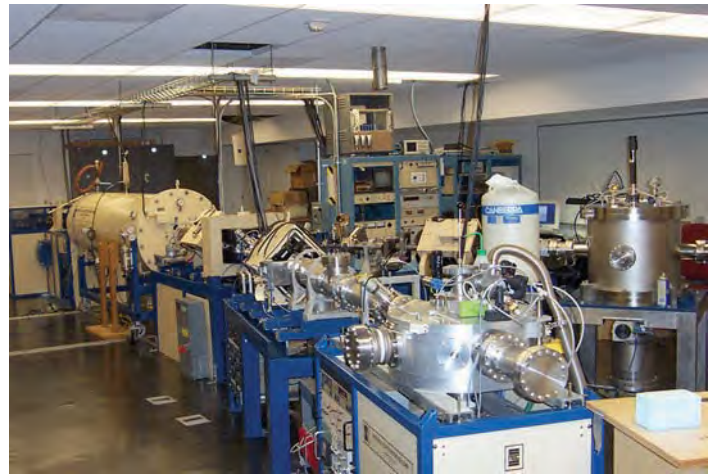
The beige cylinder in the background is the linear accelerator at the heart of the Naval Academy Tandem Accelerator Laboratory. A beam of high-speed protons travels from the accelerator to the target area in the foreground. (Gene Mosca.)
