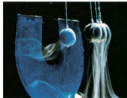
A superconductor is a perfect diamagnet. Here the superconducting pendulum bob is repelled by the permanent magnet. (© Bill Pierce/Time Magazine, Inc.)
