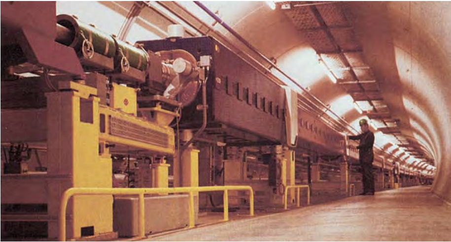
The tunnel of the proton–antiproton collider at CERN. The same bending magnets and focusing magnets can be used for protons or antiprotons moving in opposite directions. The rectangular box in the foreground is a focusing magnet, and the next four boxes are the bending magnets. (CERN.)
