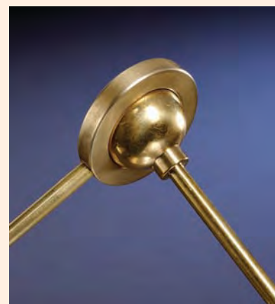
FIGURE 20-1 When the ball and ring are both at room temperature, the ball is too big to pass through the ring. The ring expands when heated, and when it is hot the ball, which remains at room temperature, is able to pass through the hole. (Richard Megna/Fundamental Photographs.)
