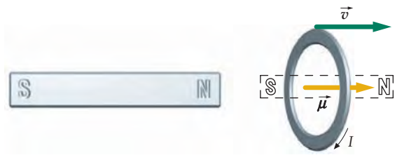
FIGURE 28-13 When the loop is moving away from the stationary bar magnet, the bar magnet attracts the magnetic moment of the loop, again opposing the relative motion.
