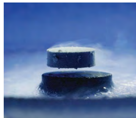
The disk is a superconductor. The magnetic levitation results from the repulsion between the permanent magnet producing the applied field and the magnetic field produced by the currents induced in the superconductor. (© Palmer/Kane, Inc./CORBIS.)
