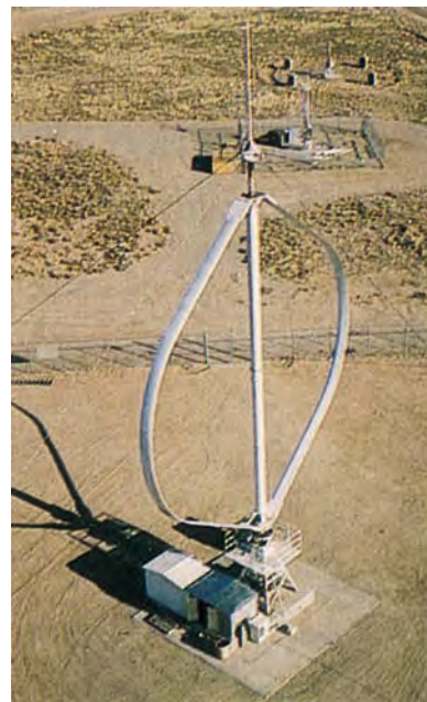
An experimental wind-powered electric generator at Sandia National Laboratory. The propeller is designed for optimum transfer of wind energy to mechanical energy. (Sandia National Laboratory.)
