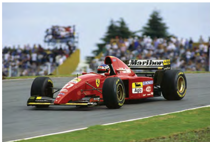
The wing on this Formula 1 racing car deflects the air upward, increasing downforce on the car for better control at high speeds. In addition, an underbody venturi reduces the pressure under the car body. The downforce associated with this pressure reduction is called the ground effect. (Schlegelmilch/Corbis.)
