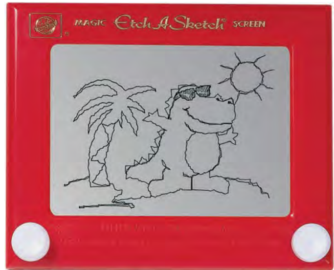
A fine powder is attracted to the back of the screen by electrostatic. Turning the knobs results in the power being rubbed off by a small stylus. (Courtesy of The Ohio Art Company.)
