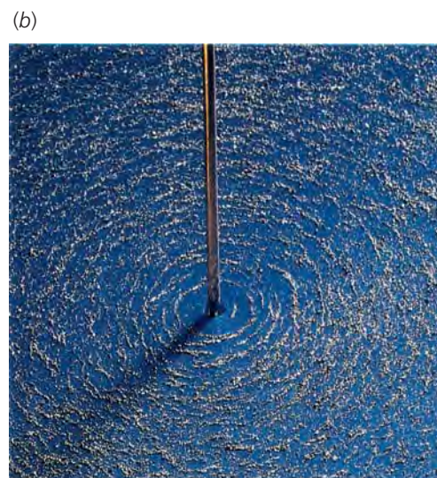
FIGURE 27-18 (a) Right-hand rule for determining the direction of the magnetic field due to a long, straight, current-carrying wire. The magnetic field lines encircle the wire in the direction of the fingers of the right hand when the thumb points in the direction of the current. (b) Magnetic field lines due to a long wire, which is indicated by iron filings. (© 1990 Richard Menga/Fundamental Photographs.)
