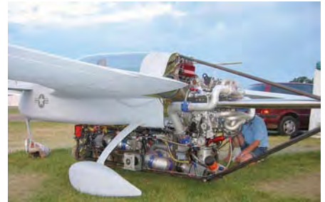
Experimental pulse detonation engine in Rutan Vari-Eze. (Tim Anderson.)
