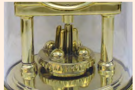
This clock keeps time by using a torsional oscillator. (Courtesy of Bill Master/Alibaba. http://yuning.en.alibaba.com .)
