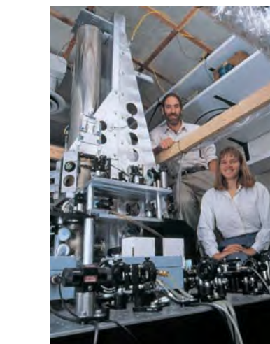
Cesium fountain clock with developers Steve Jefferts and Dawn Meekhof. (© 1999 Geoffrey Wheeler.)
