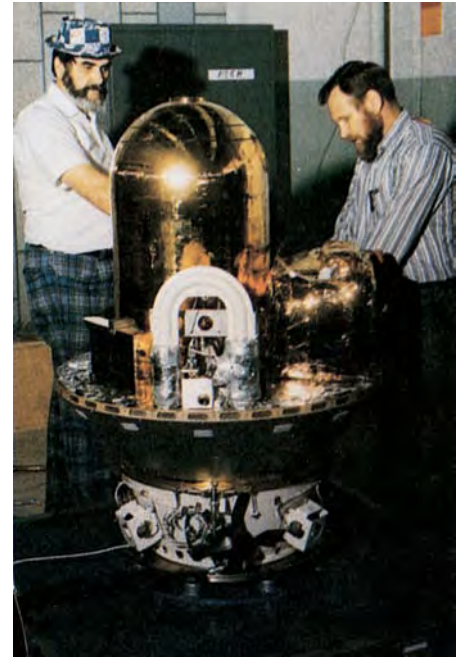
This extremely accurate hydrogen maser clock was launched in a satellite in 1976, and its time was compared to that of an identical clock on Earth. In accordance with the prediction of general relativity, the clock on Earth, where the gravitational potential was lower, lost approximately 4.3 \times 10^{-10} s each second compared with the clock orbiting Earth at an altitude of approximately 10000 km. (NASA.)
