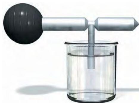
FIGURE 13-21 When the bulb of an atomizer is squeezed, the air is forced through the constriction in the horizontal tube, which reduces the pressure there below atmospheric pressure. Because of the resulting pressure difference, the liquid in the jar, which is open to the atmosphere is pumped up through the vertical tube, enters the air stream, and emerges from the nozzle. A similar effect occurs in the carburetor of a gasoline lawnmower engine.
