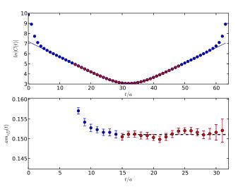
• Kaon correlation function and effective mass from RBC-UKQCD's simulation on a  $32^3 \times 64$  DWF lattice with  $a^{-1} = 2.28$  GeV.
