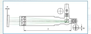
An autocollimator with geometrical beam splitter is arranged similarly (see illustration below). The collimator reticle is reflected into the beam path by the path-folding mirror which has a small angle in relation to the optical axis. The beam reflected off the target mirror passes below the path-folding mirror and produces an image of the collimator reticle in the eyepiece reticle plane.
