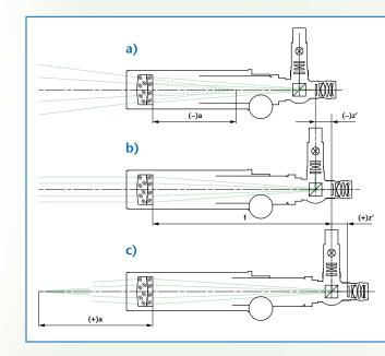
The geometrical beam splitter results in smaller image angles, but greater image brightness and less stray light. These autocollimators are used mainly with small targets. Due to their internal layout, these autocollimators cannot be used for measurement of triple mirrors or corner cubes. In most cases an autocollimator with physical beam splitter is recommended, due to the larger measuring range of this configuration. Fixed or variable distance setting?
