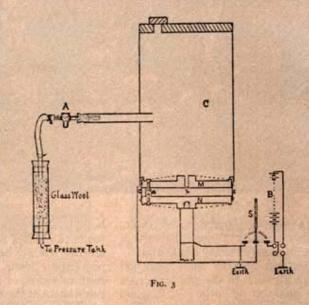
The air with which this spray was blown was first rendered dust-free by passage through a tube containing gla-s wool. The minute droplets of oil constituting the hem having dine
