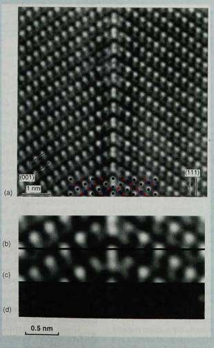
data (b), together with the atomic structure assumed in the simulation (the colored dots), which can be compared with the calculated image (c). The simulation was based on quantitative refinement, and the small residual differences—of order the experimental errors—are displayed in the bottom part of the figure (d).
