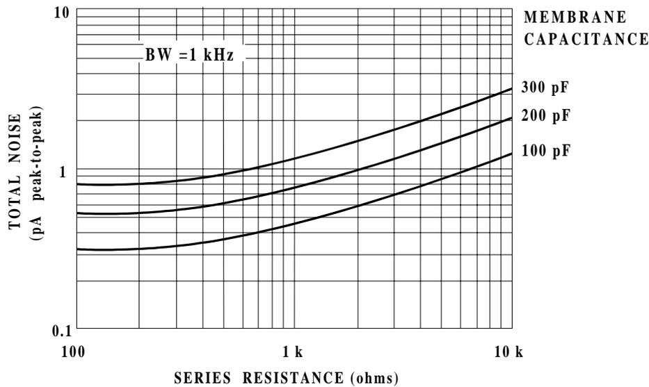
**Figure 3-25.** Typical Current Noise in Bilayer Experiments
