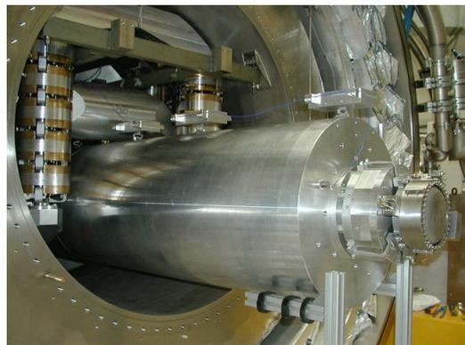
Figure 1: The AURIGA gravitational wave detector consists of a 3-meter aluminum cylinder, cooled to a few thousandths of a degree above absolute zero. The bar is kept carefully isolated from other vibrations, to help measure tiny gravitational disturbances - or possibly quantum-gravitational effects.
