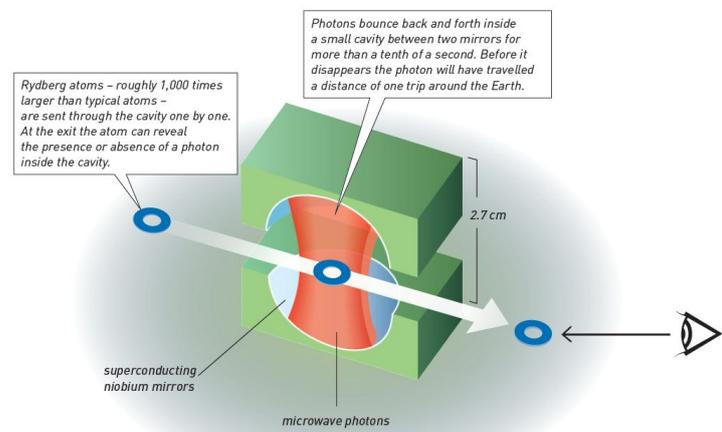
Figure 2: In the Serge Haroche laboratory in Paris, in vacuum and at a temperature of almost absolute zero, the microwave photons bounce back and forth inside a small cavity between two mirrors. The mirrors are so reflective that a single photon stays for more than a tenth of a second before it's lost. During its long life time, many quantum manipulations can be performed with the trapped photon without destroying it.
