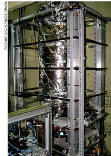
The first atomic fountain in Brazil is used for high-precision spectroscopy experiments and other studies requiring an atomic clock.
