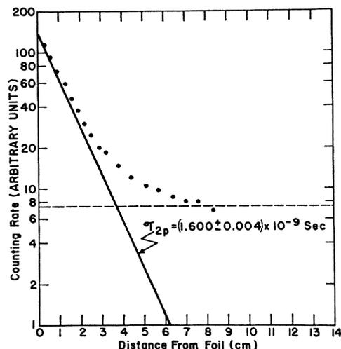
FIG. 3. Results of measurements of Lyman  $\alpha$  radiation. Solid points are experimental data. Solid straight line represents the mean life of the  $2p$  state, while the dashed line is the computer-fitted constant term.
