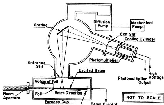
FIG. 2. Experimental arrangement showing spectrometer, target chamber, and detector chamber. Suppressor plate and grounded shield on Faraday cup are not shown.
