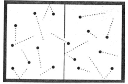
Free expansion of a gas is a thermodynamically irreversible process: one in which the entropy, or disorder, of the universe increases. A gas is initially confined in one chamber of a two-chamber apparatus (a). The barrier between the chambers is pierced, and molecules leak from one chamber into the other until approximately the same number of molecules are in both (b).
