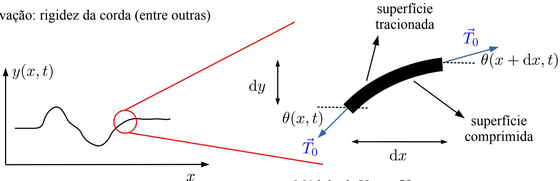
Teoria elástica:  $\rho \frac{\partial^2 y}{\partial t^2} = T \frac{\partial^2 y}{\partial x^2} - Y I \frac{\partial^4 y}{\partial x^4} = 0$
