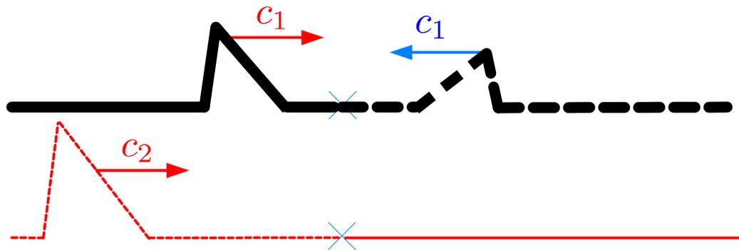
$$y(x, t) = \begin{cases} f_{\text{in}}(x - c_1 t) + g_{\text{R}}(x + c_1 t), & x < 0 \\ f_{\text{T}}(x - c_2 t), & x > 0 \end{cases}$$
