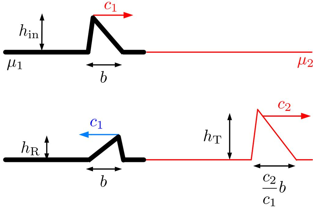
$$y(x, t) = \begin{cases} f_{in}(x - c_1 t) + g_R(x + c_1 t), & x < 0 \\ f_T(x - c_2 t), & x > 0 \end{cases}$$
