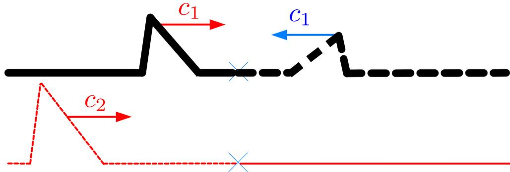
$$\frac{\partial^2 y}{\partial x^2} - \frac{1}{c_1^2} \frac{\partial^2 y}{\partial t^2} = 0 \quad \text{para } x < 0$$
