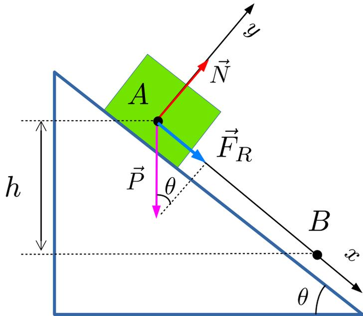
$$\begin{aligned}W_R &= \int \vec{F}_R \cdot d\vec{r} = \int (\vec{P} + \vec{N}) \cdot d\vec{r} = W_P + W_N \\ &= W_P + 0 = m\vec{g} \cdot \int d\vec{r} = m\vec{g} \cdot \Delta\vec{r} \\ &= mgAB \sin \theta = mgh\end{aligned}$$
