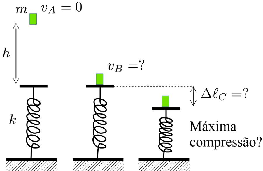
$$E_A = mgh = E_B = \frac{1}{2}mv_B^2, \quad \Rightarrow \quad v_B = \sqrt{2gh}$$
