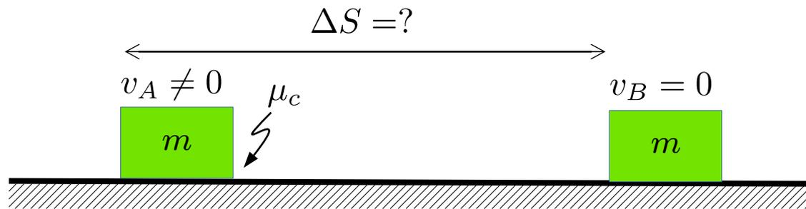
$$W_{\text{at}} = \int_{A,\Gamma}^B \vec{F}_{\text{at}} \cdot d\vec{r} = -F_{\text{at}} \Delta S = -\mu_c mg \Delta S = \Delta E_c = -\frac{1}{2} m v_A^2$$
