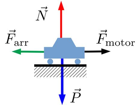
$$\vec{F}_R \approx \vec{P} + \vec{N} + \vec{F}_{\text{arr}} + \vec{F}_{\text{motor}} = \vec{0}$$
