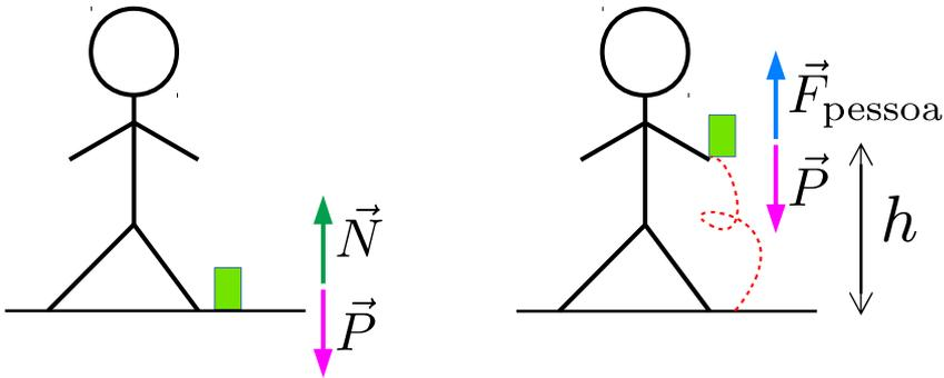
$$\begin{aligned}W_R &= \Delta E_c = 0 \\&= W_P + W_F = m\vec{g} \cdot \Delta\vec{r} + W_F \\&= -mgh + W_F, \quad \Rightarrow \quad W_F = mgh\end{aligned}$$
