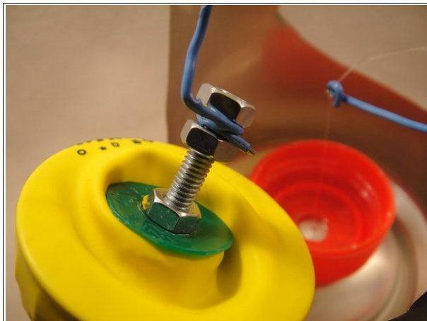
Bolt the diaphragm down
