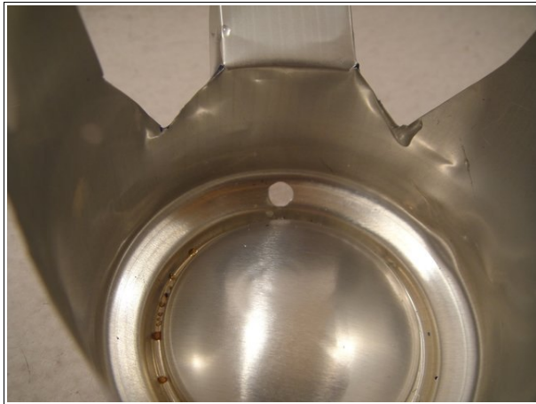
Drill a hole in the top can
