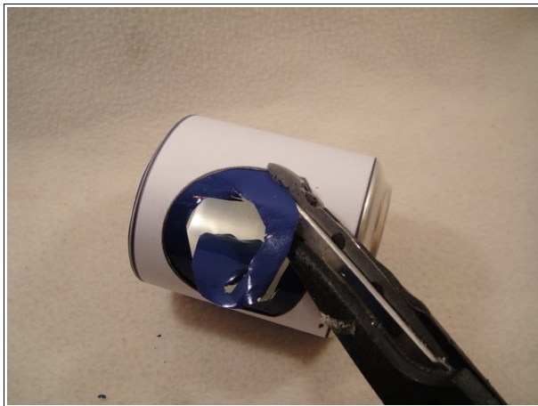
Cut around the template
