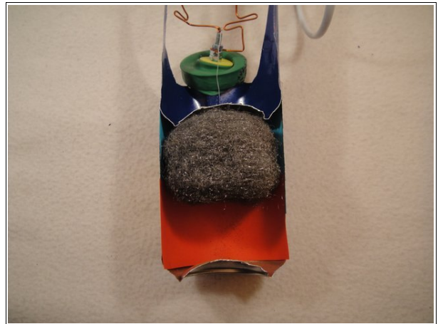
The displacer in the heating cycle
