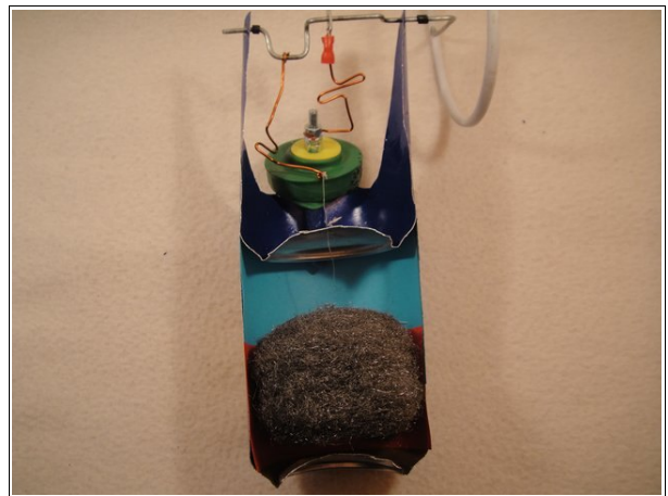
The displacer in the cooling cycle
