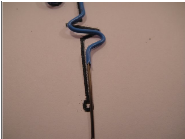
Strip the plastic off the end
