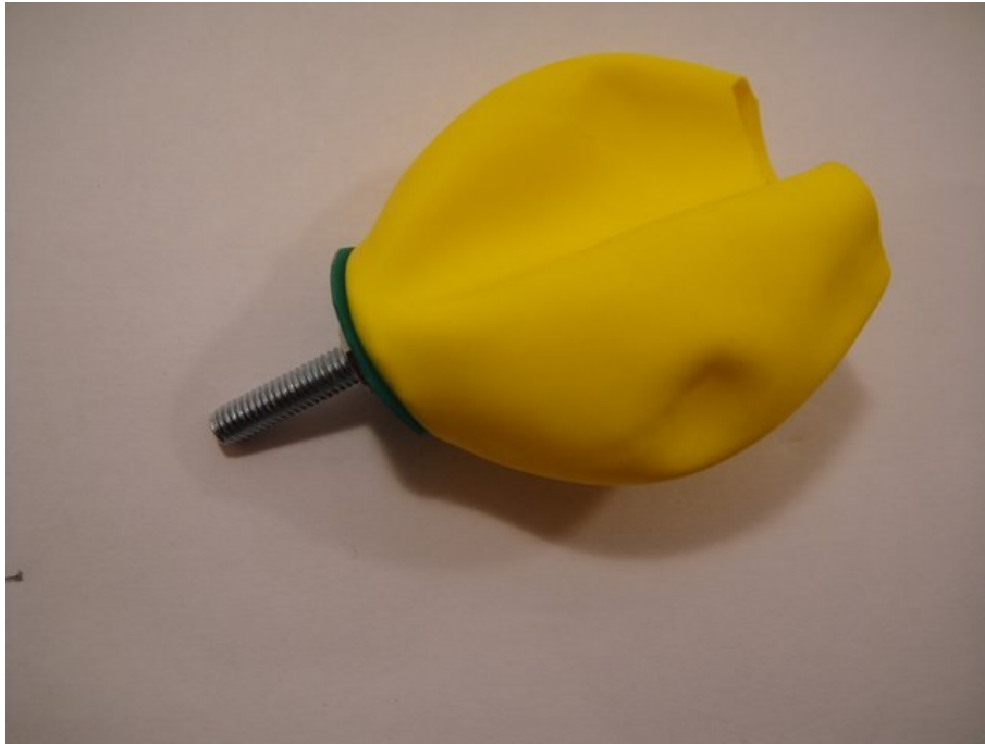
The finished diaphragm
