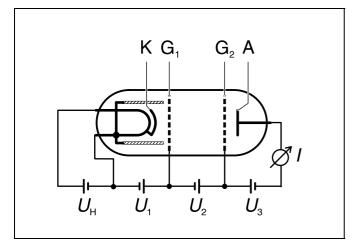
sufficient to transfer the energy required to excite the neon atoms through collisions. The collector current drops off dramatically, as after collision the electrons can no longer overcome the braking voltage  $U_3$ .
