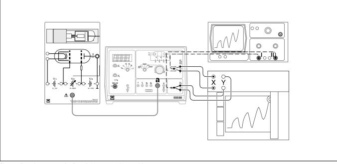
Fig. 2: Experiment setup for Franck-Hertz experiment with neon
