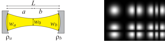
Figure 18.32: (code) (Left) Scheme of a linear cavity. (Right) Radial profiles of the lowest order transverse Hermite-Gaussian modes \text{TEM}_{mn} of a linear cavity.
