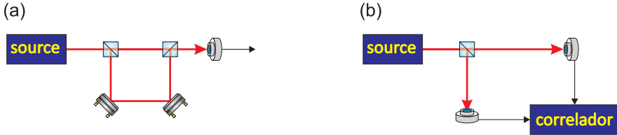
Figure 35.13: (a) Scheme of Young's experiment. (b) Scheme of the experiment of Hanbury, Brown, and Twiss. Young's experiment reveals the coherence of a field, that is, its ability to interfere. In contrast, the Hanbury-Brown-Twiss experiment reveals correlations between the (quasi-)particles constituting the field, that is, effects due to quantum statistics or interactions.
