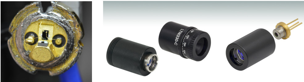
Figure 53.28: (Left) Laser diode with protective housing removed, e.g. using a can opener. (Right) Laser diode collimator.
