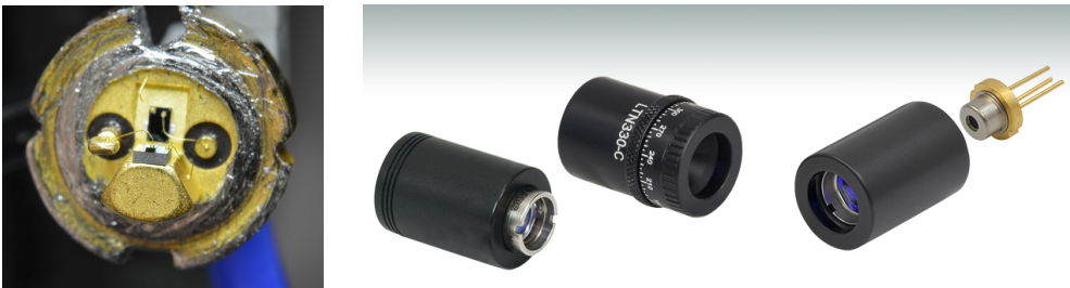
Figure 32.26: (Left) Laser diode with protective housing removed, e.g. using a can opener. (Right) Laser diode collimator.
