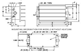
Figure 7.15: Data sheet for the rf-amplifier from MiniCircuits, model ZHL-2-8.
