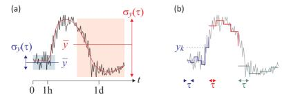
Figure 7.11: (a) Noise can exhibit very different short and long time behavior. (b) Any measurement needs a minimum integration time.
