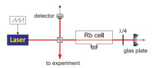
Figure 5.11: Saturation spectroscopy.
