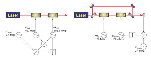
Figure 6.17: Two schemes for laser tuning.
