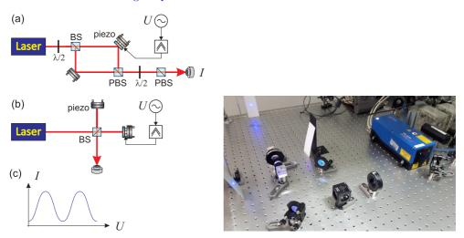
Figure 4.17: Setup for (a) a Mach-Zehnder interferometer or (b) a Michelson interferometer. (BS) non-polarizing beamsplitter, (PBS) polarizing beamsplitter. (c) Signal on the photodetector as a function of the length variation of an arm of the interferometer.
