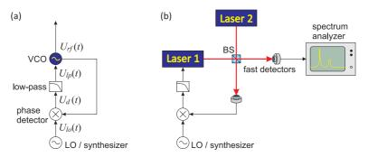
Figure 6.14: (a) PLL to lock a VCO to a reference oscillator LO. (b) PLL to lock the difference frequency of two lasers to a LO.
