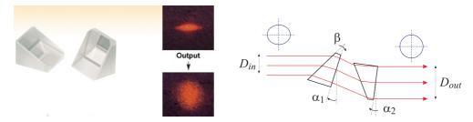
Figure 2.8: (Left) Anamorphic prisms (Thorlabs, PS870). (Right) Geometry of the beam transformation. The entrance side of a prism is often chosen close to the Brewster angle, while the exit side treated carries an anti-reflexion coating.
