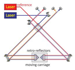
Figure 5.4: Principle of operation of a Michelson-type wavemeter.
