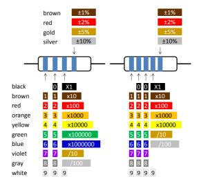
Figure 3.1: Color code for resistors with 4 and 5 rings.
