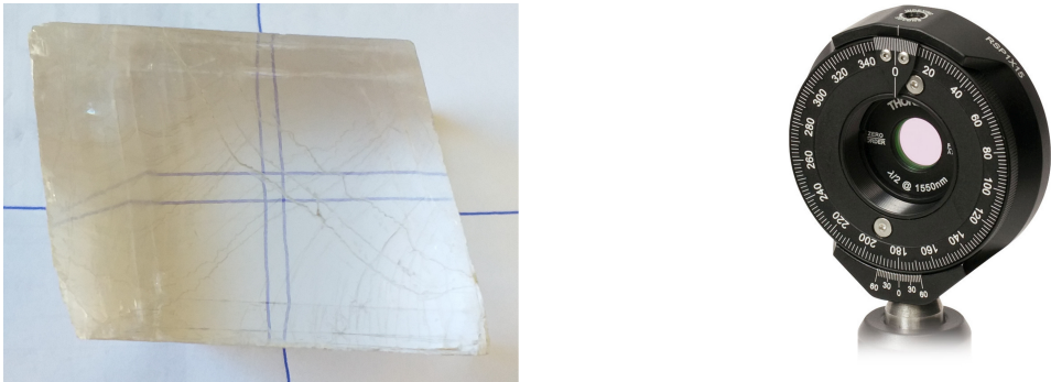
Figure 2.7: (Left) Transmission through a birefringent crystal. (Right) \lambda/2 -waveplate mounted in a rotation stage.
