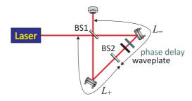
Figure 4.16: Double Mach-Zehnder interferometer.
