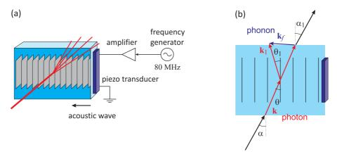
Figure 4.32: (a) Principle of the acousto-optic modulator. (b) Scheme of the diffraction in an acousto-optic modulator: A photon with wavevector k is scattered by a phonon with wavevector  $k_1$  resulting in a photon with wavevector  $k_f$ .
