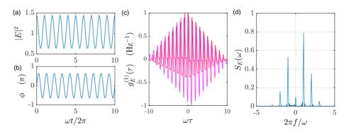
Figure 4.4: (code) (a) Amplitude and (b) phase of the electric field, with n=0.2, m=1, and  $\omega_n=\omega_m=(2\pi)$  1 Hz. (c) Aurocorrelation function and (d) spectrum of the light field.
