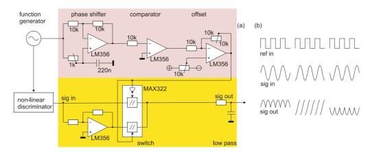
Figure 3.17: (a) Principal scheme of a lock-in amplifier. (b) Mode of operation.
