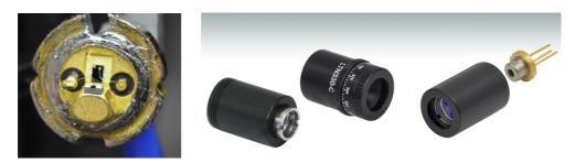
Figure 4.26: (Left) Laser diode with protective housing removed, e.g. using a can opener. (Right) Laser diode collimator.
