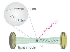
Figure 1.10: (code for download) Two-level atom interacting with a cavity mode.
