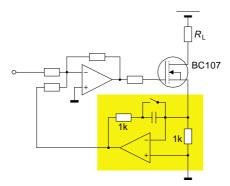
Figure 6.7: Current stabilization.
