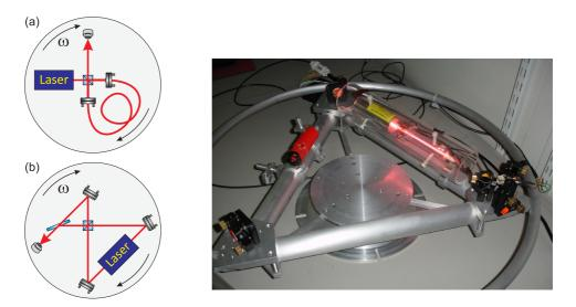
Figure 4.10: (a) Principle scheme of a fiber-based Sagnac interferometer. (b,c) Laser gyroscope realized with a HeNe gain tube.
