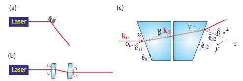
Figure 2.9: Beam steering with two rotatable wedged substrates (see Thorlabs, PS810).
