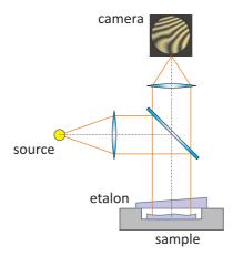
Figure 4.19: Principle of operation of a Fizeau interferometer.
