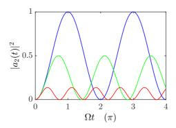
Figure 1.9: (code for download) Probability  $|a_2(t)|^2$  for the atom to be in the excited state for  $\Omega = \Gamma$  and  $\Delta = 0$  (blue),  $\Delta = \Gamma$  (green), and  $\Delta = 2.5\Gamma$  (red). Time is in units of  $1/\Gamma$ .
