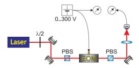
Figure 2.15: Scheme for using an EOM as a Pockels cell.
