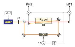
Figure 5.8: Schemes of frequency-modulation and modulation transfer spectroscopy.
