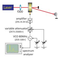
Figure 4.38: Setup for testing an acousto-optic modulator.
