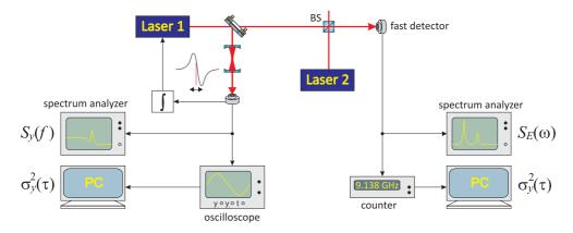
Figure 7.12: (left) Setup for measuring the spectral density of frequency fluctuations  $S_y(f)$  and the Allan variance  $\sigma_y^2(\tau)$  of laser 1 discriminating it at the slope of transmission signal of an optical cavity. (right) The power spectral density  $S_{\mathcal{E}}(\omega)$  can be found as the beat signal between two lasers and either be exhibited on a spectrum analyzer  $S_{\mathcal{E}}(\omega)$  or counted and processed to an Allan variance  $\sigma_y^2(\tau)$ .
