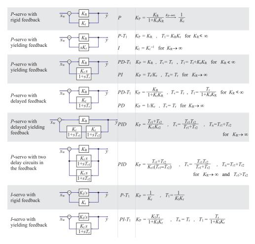
Figure 7.8: Some examples for feedback regulators. The columns show from left to right: the nomenclature, the circuit diagram, the behavior, and the constants of the LTI system.
