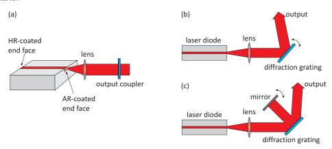
Figure 4.28: (a) ECDL with an AR-coated laser diode and an external mirror. (b) Littrow configuration. (c) Littmann configuration.
