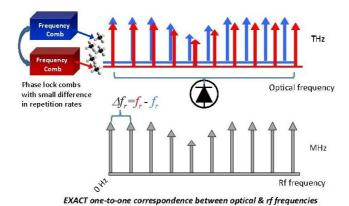
Figure 5.17: Principle of dual comb spectroscopy.
