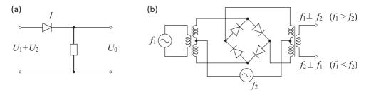
Figure 3.15: (a) Mixing two signal at a diode. (b) Schematic diagram of a double-balanced passive diode mixer (also known as a ring modulator). There is no output unless both  $f_1$  and  $f_2$  inputs are present, though  $f_2$  (but not  $f_1$ ) can be DC.
