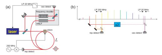
Figure 5.16: (a) Scheme and (b) operation principle of a frequency comb with control of the repetition rate and the carrier envelope offset.
