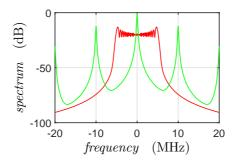
Figure 3.14: (code) Frequency spectra of a phase-modulated carrier frequency for  $\Delta\omega=5\,\mathrm{MHz}$  modulation excursion and (red)  $\omega=100\,\mathrm{kHz}$  modulation frequency ( $\beta=\frac{\Delta\omega}{\Omega}=50$ ) and (green)  $\omega=10\,\mathrm{MHz}$  modulation frequency ( $\beta=0.5$ ). Furthermore, a  $\gamma=100\,\mathrm{kHz}$  resolution linewidth is assumed.
