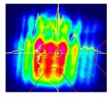
Figure 4.27: Typical beam profile of a multimode laser diode (Thorlabs, L450P1600MM.
