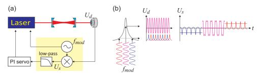
Figure 6.10: (a) Frequency stabilization to a cavity using the lock-in method. (b) Frequency-modulated signals applied to a resonance suffer a period doubling, when the signal frequency is close to resonance. By demodulating the signals discriminated at the resonance profile, we obtain, after averaging over a period, a DC voltage that is proportional to the frequency detuning. The yellow area denotes the components constituting the lock-in amplifier.
