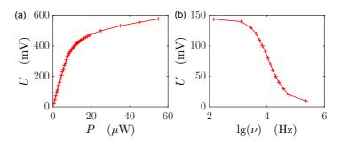
Figure 3.13: (a) Calibration of a photodiode, measured voltage as a function of the incident light power. (b) Low-pass behavior of a resistive charge of  $90 \,\mathrm{k}\Omega$ .
