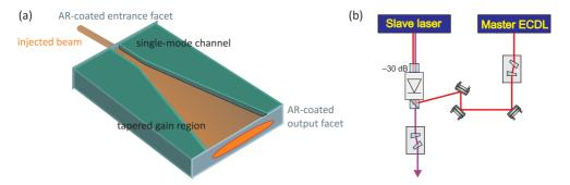
Figure 4.31: (a) Tapered amplifiers are available e.g. from Eagleyard. (b) Principle of injection locking.
