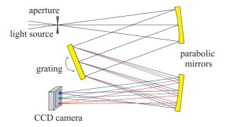
Figure 5.3: Principle of operation of a Czerny-Turner monochromator.
