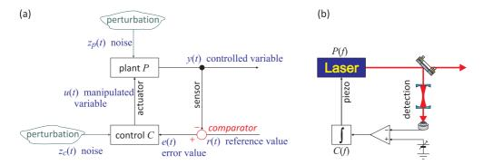
Figure 6.1: (a) General schematic diagram of a feedback loop. (b) Possible implementation for the frequency stabilization of a laser to a cavity resonance,
