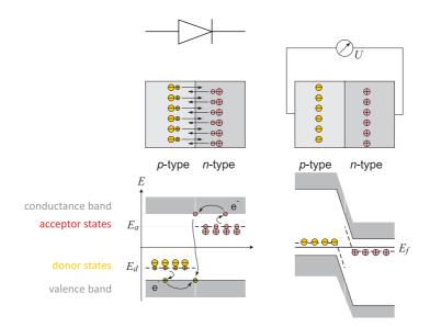
Figure 3.10: Joining a p-type and a n-type doped semiconductor (left) one observes a charge carrier redistribution across the pn transition (right).
