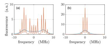
Figure 4.36: (code) Phase modulation sidebands with high (left) and low (right) modulation index resolved by a narrow (red) or broad (blue) filter.
