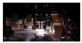
Figure 4.30: (Left) Construction plan of a home-built ECDL lasers in cat-eye configuration. (Right) Side view of the cat-eye laser.
