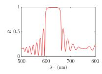
Figure 4.7: (code) Reflection by a high reflecting mirror made of 10 layers with  $n_1 = 2.4$  and  $\Delta z_1 = 80$  nm alternating with 10 layers with  $n_2 = 1.5$  and  $\Delta z_2 = 500$  nm. The absorption coefficient for each layer is supposed to be  $\alpha = 0.2\%$ . The beam impinges from vacuum,  $n_0 = 1$ .
