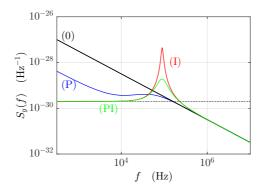
Figure 6.4: (code) Spectral density of frequency fluctuations of the servo system exhibited in Fig. 6.2. Shown is the spectral noise density  $S_y(f)$  of the laser light for 4 different feedback gain curves: (black solid) no feedback control C(f) = 0, (blue) P-regulator with C(f) = 4, (red) I-regulator with  $C(f) = 5 \cdot 10^6/if$ , and (green) PI-regulator  $C(f) = 4 + 5 \cdot 10^6/if$ .
