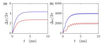
Figure 6.15: (code) Simulation of (a) the phase and (b) frequency difference in a PLL for (red)  $\omega_{lo} - \omega_0 = (2\pi)$  2 kHz and (blue) 4 kHz.
