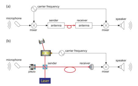
Figure 4.40: Analogy between radio transmission (a) and heterodyne techniques with a laser (b).
