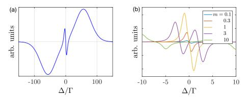
Figure 5.9: (code) (a) Calculated FMS signals and (b) MTS signals as a function of detuning for various modulation indices.
