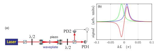
Figure 5.13: (code) (a) Generating a Hänsch-Couillaud error signal by transmission of a birefringent linear cavity. (b) Signals recorded by the two photodetectors (blue and green) and their difference (red).
