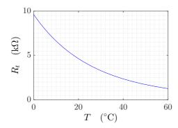
Figure 3.9: Calibration curve for a  $10 \,\mathrm{k}\Omega$  thermistor from Thorlabs.
