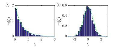
Figure 7.2: (code) (a) Boltzmann distribution simulated by random numbers (histogram). The numerical derivative of this distribution is shown as a blue dotted line, and the probability density as a green solid line. (b) Error function probability distribution simulated by random numbers (histogram). The numerical derivative of the error function is shown as a blue dotted line, and the Gauss function as a green solid line.
