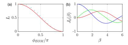
Figure 4.35: (code) (a) Effect of a Pockels cell. The solid line was calculated with the Eq. (4.60), the dotted was measured experimentally. (b) Lowest-order Bessel functions.
