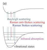
Figure 5.18: Energy-level diagram showing the states involved in Raman spectra.
