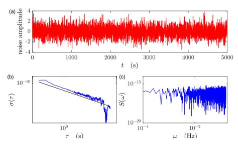
Figure 7.13: (code) Allan variance (b) and spectral density of frequency fluctuations (c) calculated from a randomly generated data set (a).
