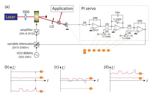
Figure 6.6: (a) Layout of the intensity control. The variable attenuator controls the amplitude of the radiofrequency driving the AOM: low voltage (0 V) increases the attenuation, high voltage (+16 V) reduces it. The sketched control circuit realizes a negative feedback, when the photodetector produces a positive signal. (b-d) Signals recorded at the test points of the circuits shown in (a). See text for explanations.
