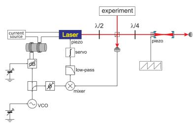
Figure 6.19: Setup of a frequency regulator following Pound-Drever-Hall. VCO: Voltage-Controlled Oscillator, LT: power splitter, dB: variable attenuator, LP: low-pass filter.
