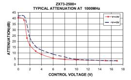
Figure 7.17: Data sheet for the voltage-controlled variable attenuator from Minicircuits, model ZX73-2500+.
