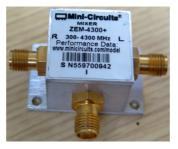
Figure 3.16: Picture of a radiofrequency mixer.
