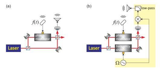
Figure 4.42: Principle scheme of the (a) homodyning and (b) heterodyning technique at the example of a Mach-Zehnder interferometer. The components in the yellow area of (b) constitute a Lock-In amplifier.
