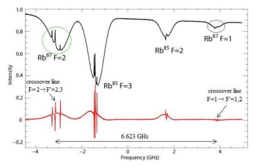
Figure 5.12: (Black) Lamb-dip spectroscopy of a rubidium gas (natural isotope mixture of <sup>85</sup>Rb and <sup>87</sup>Rb) showing the hyperfine structure transitions of the D2-line. (Red) Derivative of the spectrum in (a).
